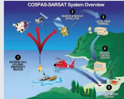
Beacons with 406Mhz, 121Mhz and GPS technologies signal for rescue from far away
