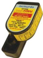
BreaktHRU hydrostatic release unit (HRU) located inside the automatic housing has a plastic bolt that secures the EPIRB to the casing, and upon activation is cut to deploy the beacon
